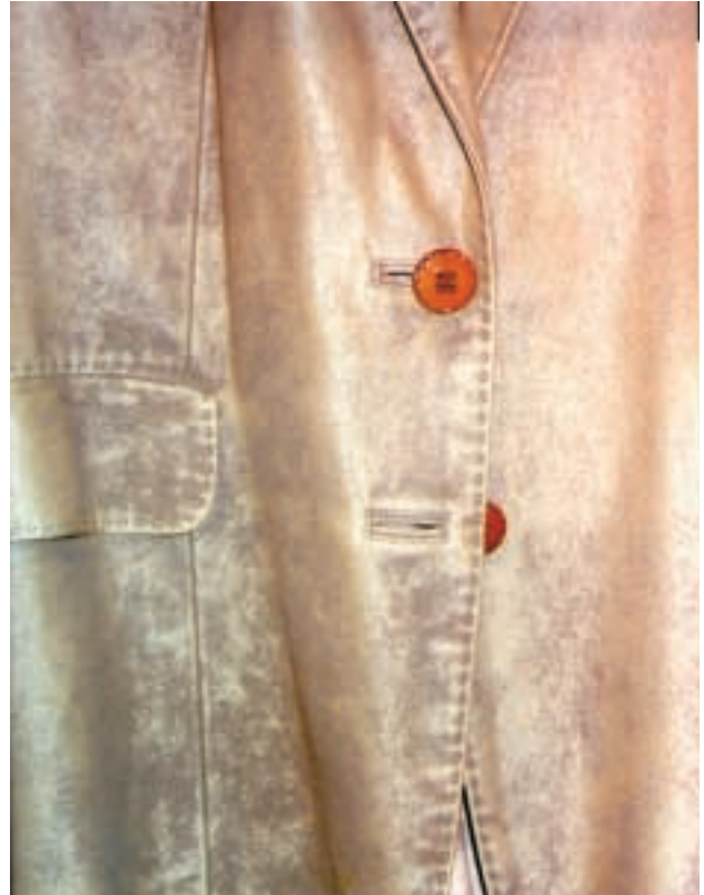
The synthetic suede finish is coming off this sport jacket from normal use and later cleaning.
